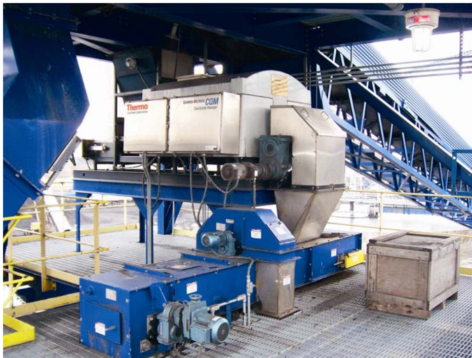
Figure 5 Thermo Scientific Coal Quality Manager (CQM TM ) is located downstream of the plant, and its ash readings enable the shift operator to vary the prep plant bypass to keep ash consistently on target.
